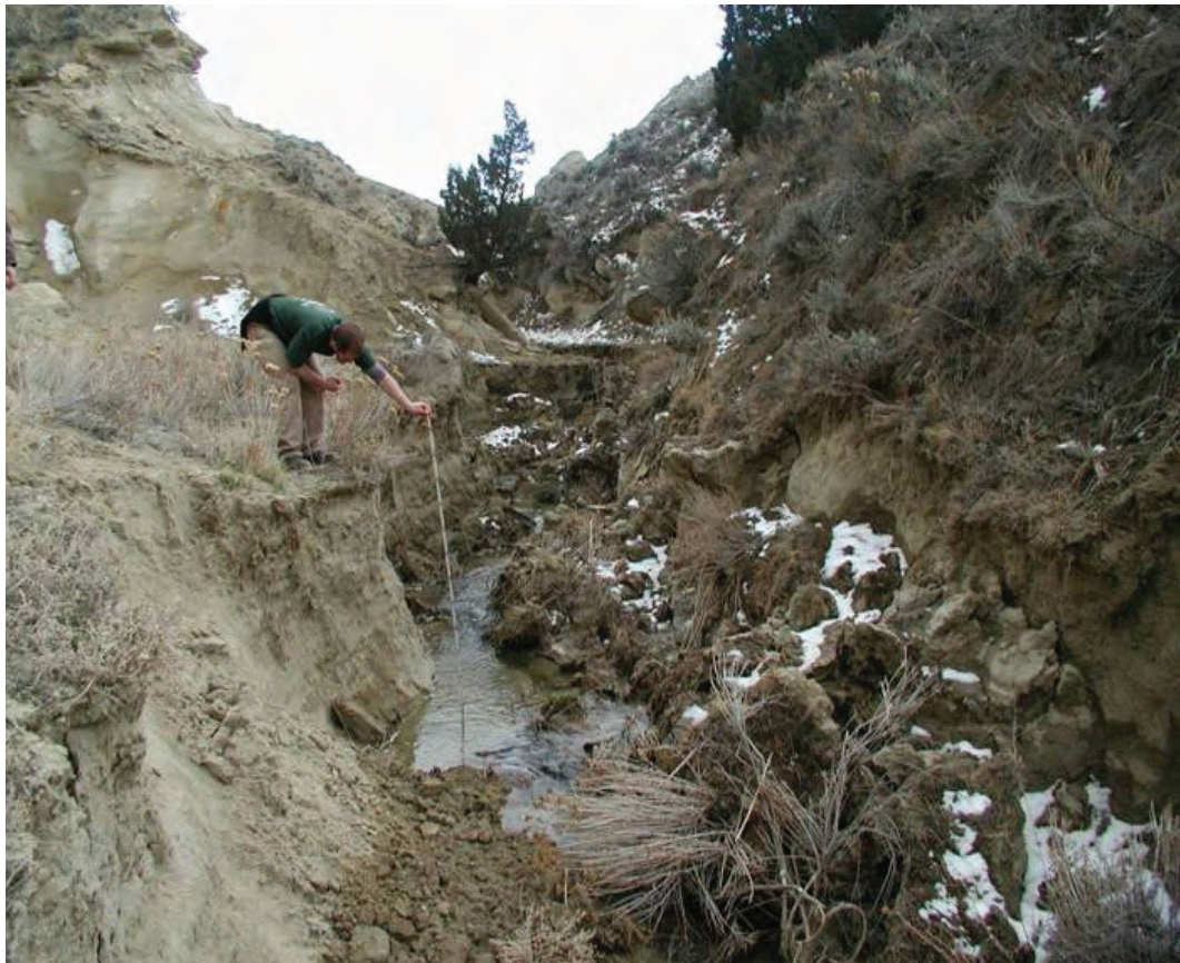
FIGURE 5.6 Stream bank erosion caused by headwater flows in ephemeral drainage of Barber Creek, Wyoming; water sourced from upgradient CBM storage impoundment releases, Powder River Basin. SOURCE: Used with permission from Gregory Wilkerson, Southern Illinois University Carbondale.
